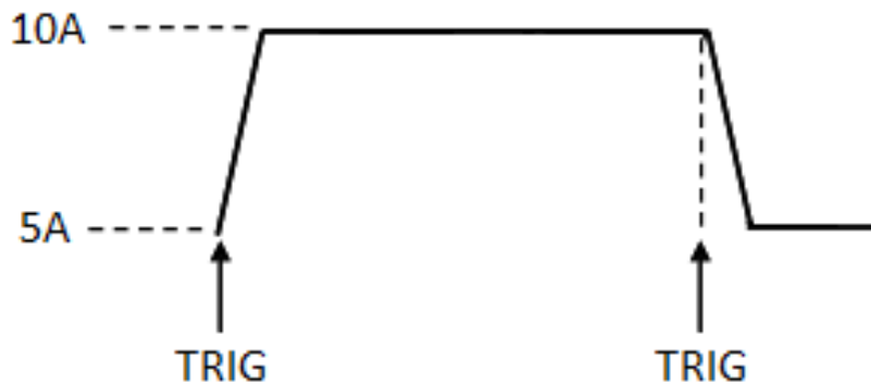
Figure 27 - Toggle Transient Operation
