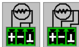
Figure 2.7: 2 and 3 wire measurement connections
