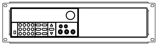
To rack mount a single instrument, order rack mount kit IT-E151
