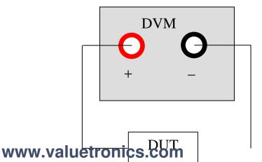
By default, the power supply is in DVM mode. Press Shift followed by  $V/m\Omega$  to toggle between Voltmeter and  $m\Omega$  Meter mode.
