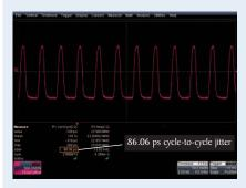
For applications requiring high signal integrity and edge stability, the 4060 Series can generate pulses with a low cycle-to-cycle jitter of < 100 ps.
