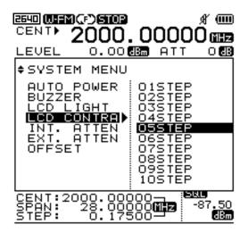
The function of LCD contrast is to adjust the contrast for the remained battery capacity.
