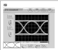
Add externally: For example long coax cable length, or Bessel-Thompson 4th Order Filter with –3 dB point at 0.75 of Bit Rate etc.
