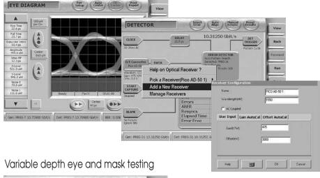
An external optical receiver may be added to the input of the BERTScope detector. Through the user interface it is easy to input and save the characteristics of the receiver. Once accomplished, relevant units on physical layer displays are changed to optical power in dBm,  $\mu W$  or mW. Coupling may be AC or DC, and the software steps the user through dark calibration.
