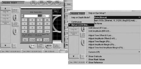
For eye diagrams and mask testing, the depth of test may be varied in manual mode; the instrument will take the specified number of waveforms then stop. The range is 2,000 to 1,000,000 bits (complete waveforms). Alternatively, the default mode is Continuous, and the eye or mask test increases in depth over time.
