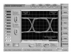
The live data option is designed to measure parametric performance of traffic that is either unknown or non-repeating. This can include traffic with idle bits inserted such as in systems with clock rate matching. It is also suitable for probing line cards, etc.
