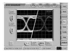
CleanEye is an eye diagram display mode, which averages waveform data to present an eye diagram with the non-data dependent jitter removed. This allows the user to view and measure data dependent jitter such as Inter Symbol Inference, giving an intuitive idea of the compensatable jitter present, for example. It is effective on any repeating pattern up to 32,768 bits long.
