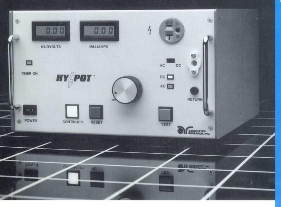
The 4450DT is our newest hipot tester. If you require both AC and DC output, in a single tester that can do all U.L. tests, this is the unit for you. For greater accuracy, the 4450DT has both a digital kilovoltmeter and a digital milliammeter, no analog meters are used.
