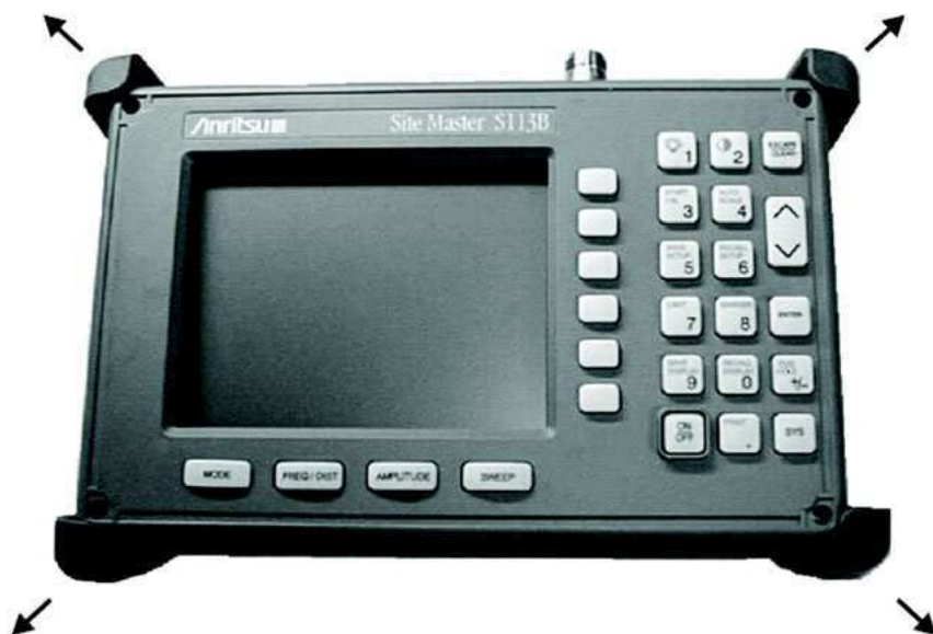
Figure 3-3. Remove the Corner Bumpers
