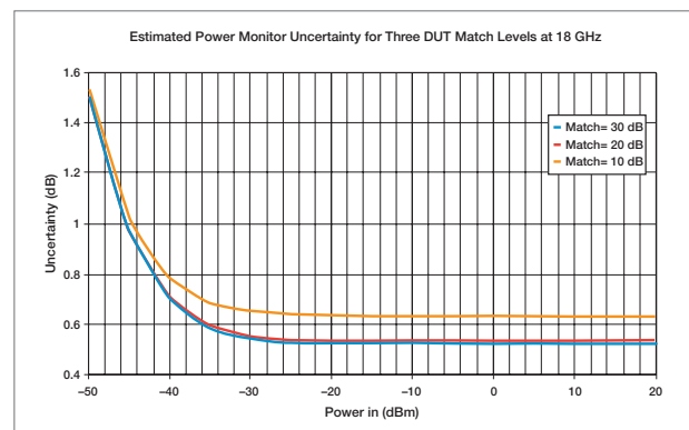
Estimated Power Monitor Uncertainty for Three DUT Match Levels at 18 GHz
