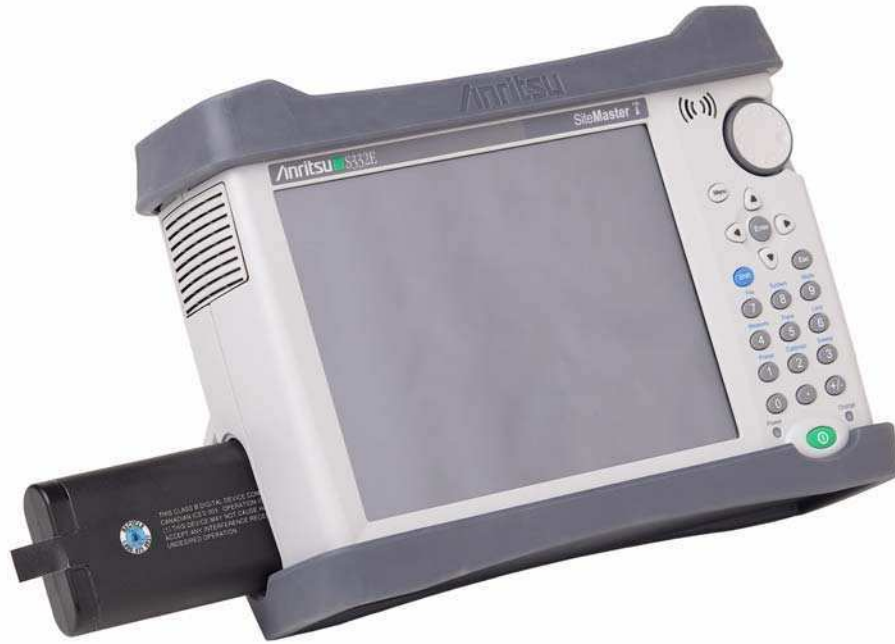
Figure 6-3. Removing the Battery
