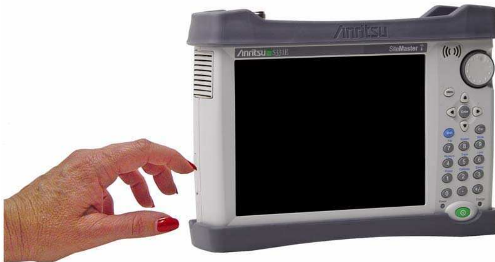
Figure 6-2. Opening the Battery Access Door
