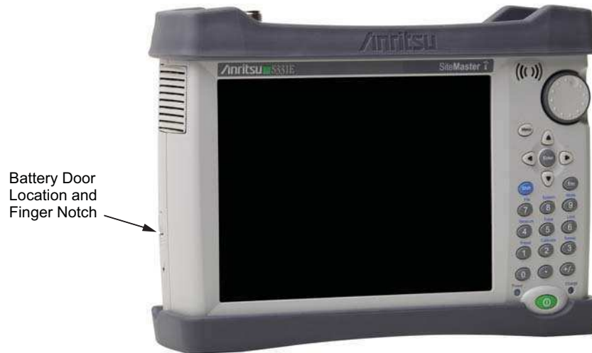
Figure 6-1. Battery Access Door Location and Finger Notch
