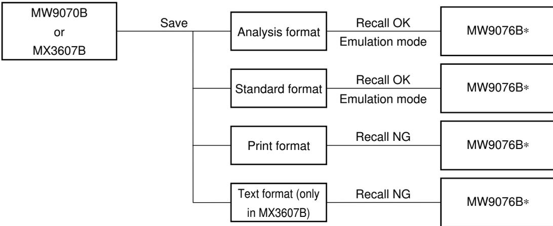
5. Among the recalled files, only the analysis format and Standard format files measured using MW9076 Series and the analysis format files measured using MW9070B can be used the event-point detection with re-auto search. Standard format files which are measured using OTDRs produced by other companies cannot be used for event-point detection even if auto search is performed.
