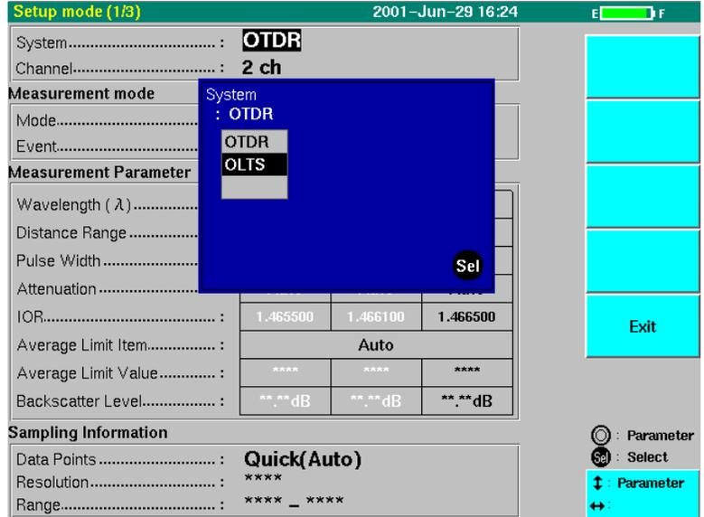
When OLTS is selected and is pressed, the system enters the OLTS measurement mode.
