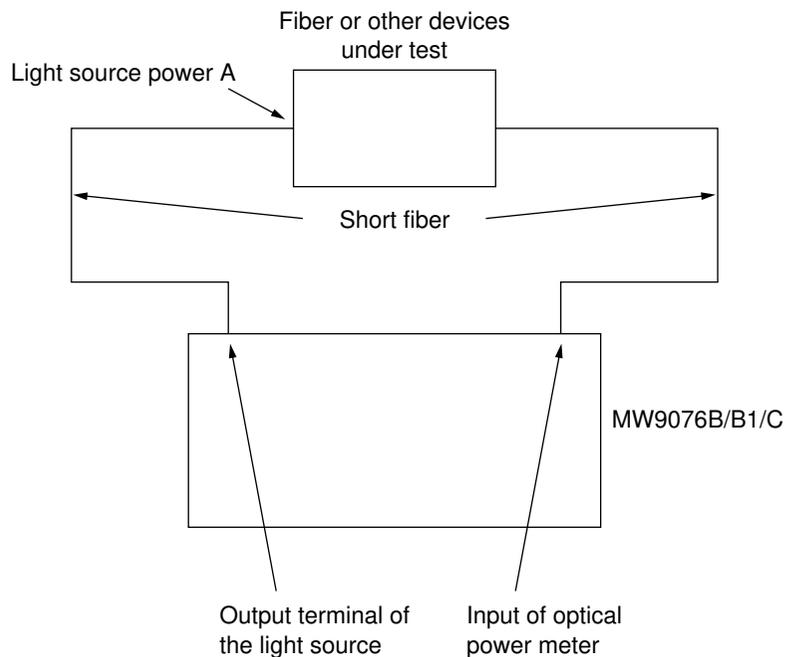
The reference value, absolute value, and loss are displayed in this order on the lower half of the OLTS screen. The loss is calculated by subtracting the absolute value from the reference value.
