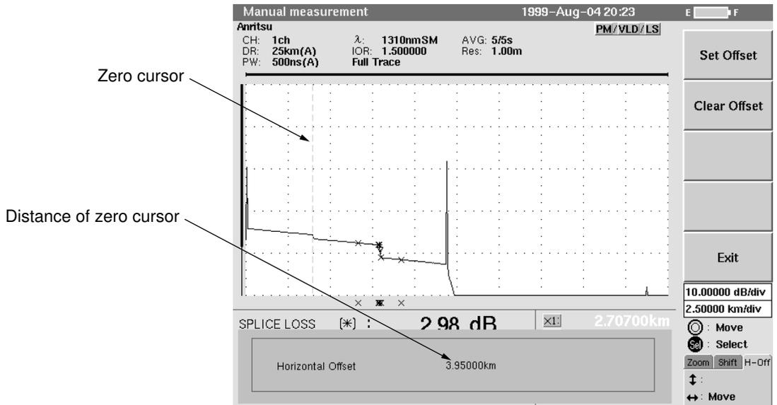
The zero cursor can be moved with the **<** and **>** keys or the rotary knob and its position is set by pressing **F1** (Set Offset).
