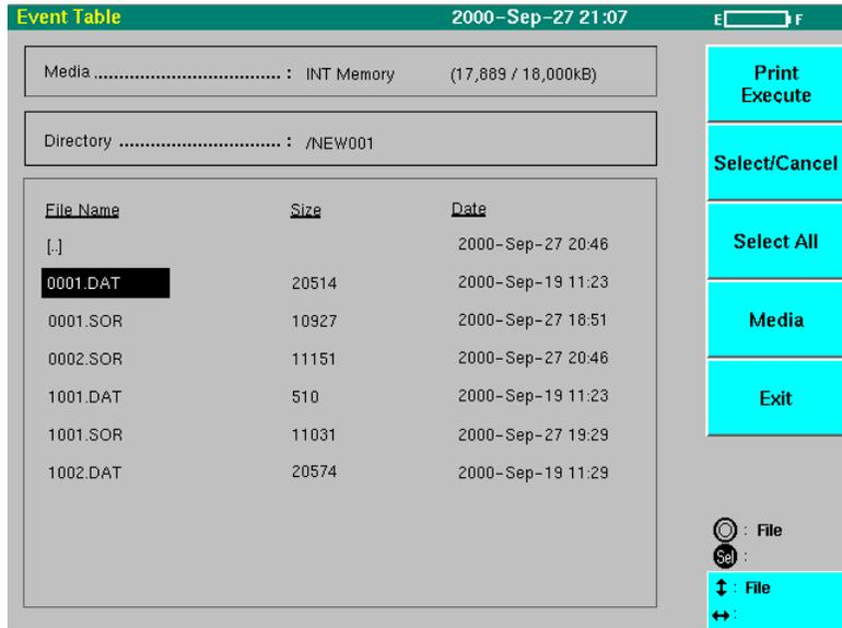
After selecting the file to be printed, press **F1** (Print Execute) to set the print details. Setting printing contents is the same as ordinal printing. See section 7.1.1 “Printing” for details.
