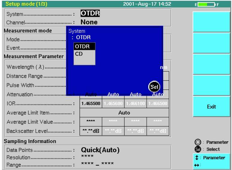
Select CD to move to the chromatic dispersion (CD) measurement. A screen appears as shown in the figure below.
