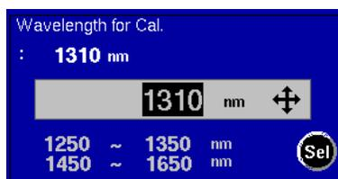
Each wavelength can be calibrated in the following wavelength ranges:
