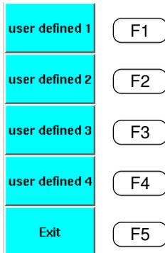
The function key label display on the left is in a state where the function names are not registered.
