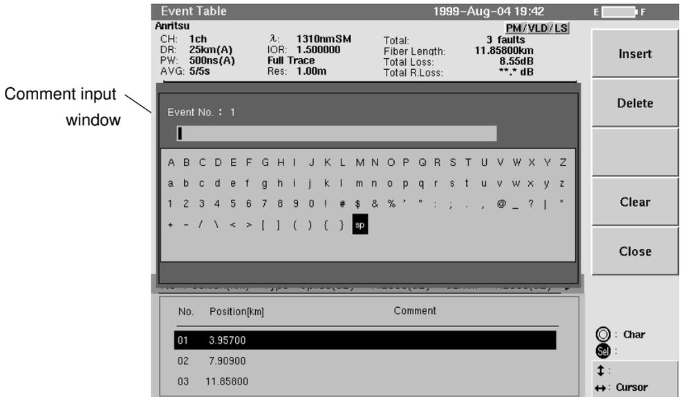
Enter a comment by selecting the characters with the rotary knob and by moving the cursor with the  $\langle$  and  $\rangle$  keys.
