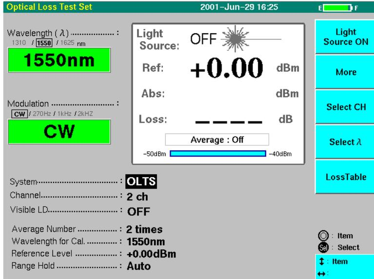
When the optional Optical Power Meter is not mounted, the screen is displayed to enable light source function operations only. MW9076B1 disables the transition to the OLTS measurement when the optical power meter is not mounted.
