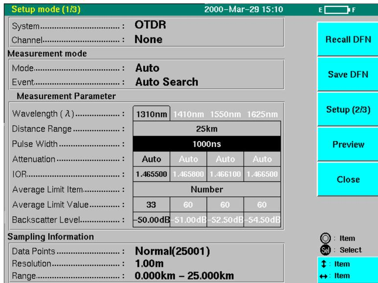
There is a possibility of OTDR failure if Setup screen 1 does not appear after the power is turned on. In this case, turn off the power and contact Anritsu Corporation or your nearest service representative.
