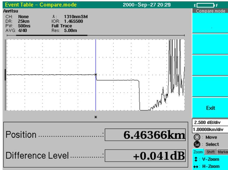
To return from the waveform difference screen to the waveform comparison screen, press **F5** (Exit).
