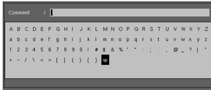
Use the **<** and **>** keys to move the cursor to the place where you want to input. Use the rotary knob to select the character you want to input. When you complete the input, press **F5** (Close). The input comment is determined and displayed next to "Comment" on the screen.
