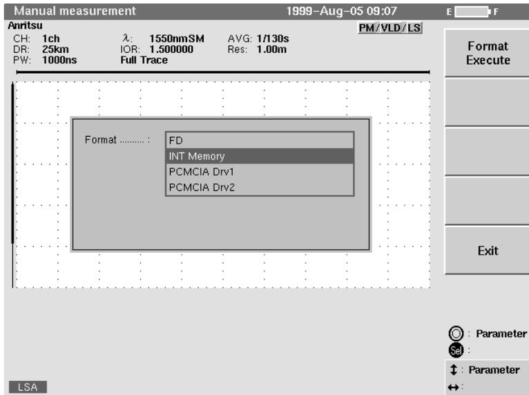
Place the cursor on the media to be initialized with the **^** and **v** keys or the rotary knob.
