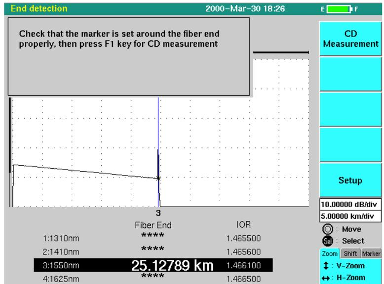
In the Auto mode, pressing **F2** (Select  $\lambda$ ) during a measurement stops the measurement using the wavelength measured and causes the OTDR measurement using the next wavelength to be resumed. Pressing **F2** during a measurement using the wavelength of 1625 nm causes the measurement to be resumed using the wavelength of 1310 nm.
