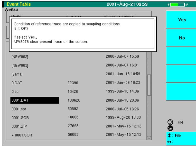
To measure using the same conditions as the selected waveform, press **F1** (Yes). The selected file is read as the reference waveform and also the current waveform for MW9076.
