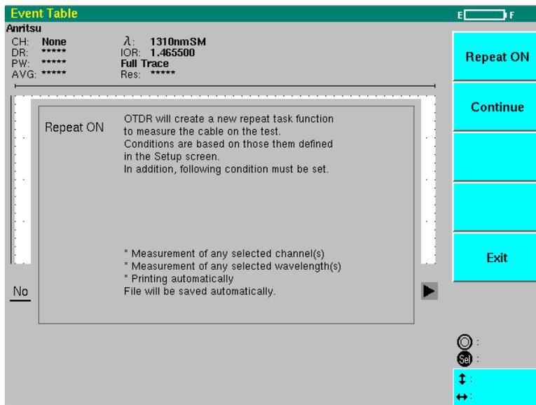
Press **F1** (Repeat ON) here to delete the previously recorded log table and to create a new log table. Afterward, move to the measurement condition setting screen of repeat task as described later.
