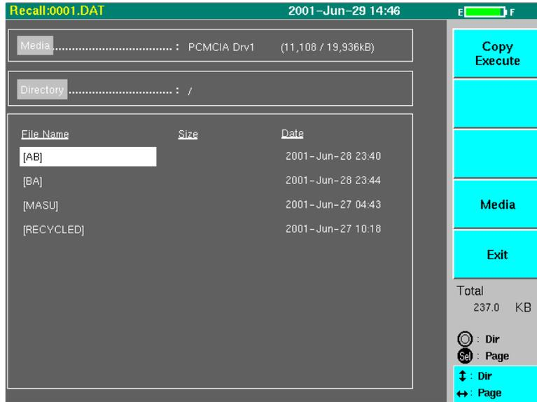
Select the media of copy target by using **F4** (Media) and select the directory by using the **^**, **v**, **<** and **>** keys.
