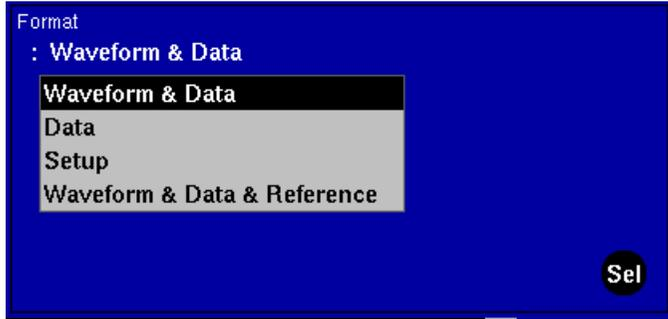
Place the cursor on the format to be set using the  $\wedge$  and  $\vee$  keys.
