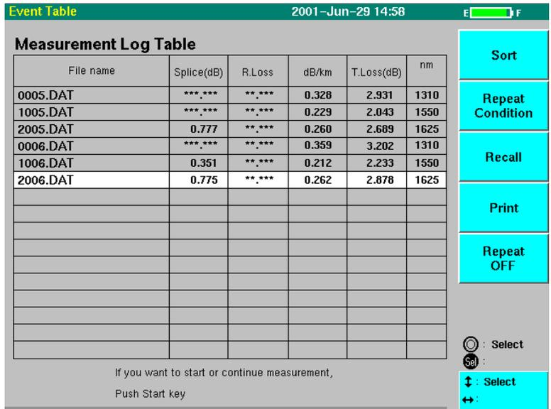
In the measurement log table, the measured data is controlled for each file name and the maximum value of each measurement result is displayed. Splice Loss, Return Loss, Fiber Loss (dB/km), Total Loss, and wavelength are displayed as measurement results (see the figure above).
