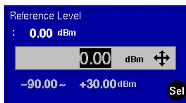
By pressing **F3** (Abs → Ref) during the measurement, the absolute value at that time is set as the reference level. **F3** (Abs → Ref) can be selected by using **F2** (More).
