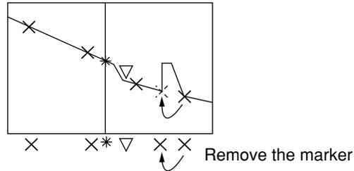
**4.12.4 Measuring the connection loss (connector)**
