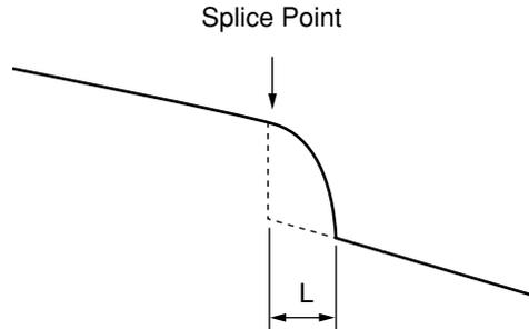
Therefore, the splice loss cannot be measured correctly in the Loss mode. In the Splice & Return Loss mode, two markers are set on each side of the splice point. The splice loss is calculated as shown below.
