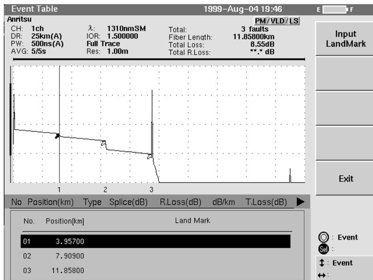
Select the event using the rotary knob or the arrow  $\uparrow$   $\downarrow$  keys. The pages can be changed using the arrow  $\leftarrow$   $\rightarrow$  keys. Three events are displayed on one page.
