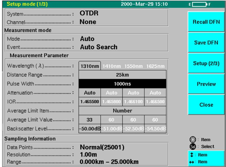
If **F2** (Save DFN) is pressed when the Setup screen 1 is displayed, the function key labels are changed as shown below.
