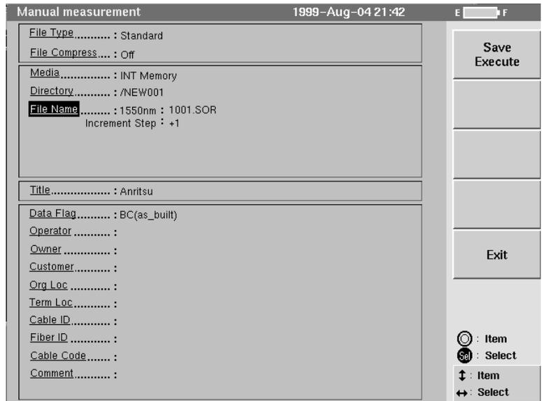
Place the cursor on the desired item with the  $\uparrow$  and  $\downarrow$  keys or the rotary knob, and then select the item with **Select** or the  $\leftarrow$  and  $\rightarrow$  keys.
