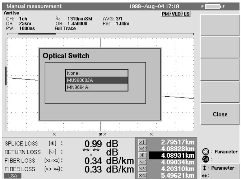
Place the cursor over the name of the optical channel selector type. The selected optical channel selector type name can be entered by pressing **F5** (Close) with the cursor placed over it.
