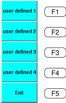
The function key label display on the left is in a state where the function names are not registered when the DFN file is saved. (For the registration of a function name, refer to “Section 3.4.2 Saving the DFN file.” If a function name is registered, the function name is displayed on each function key label.
