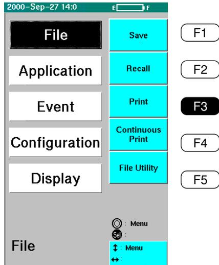
Press **F3** (Print). The printed setting screen is displayed. (See the figure below.)
