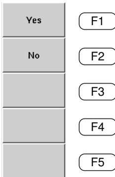
If any of the User Defined keys 1 to 4 is selected, the function keys on the left are displayed and the confirmation message “Recall user defined measurement condition. OK?” is displayed.
