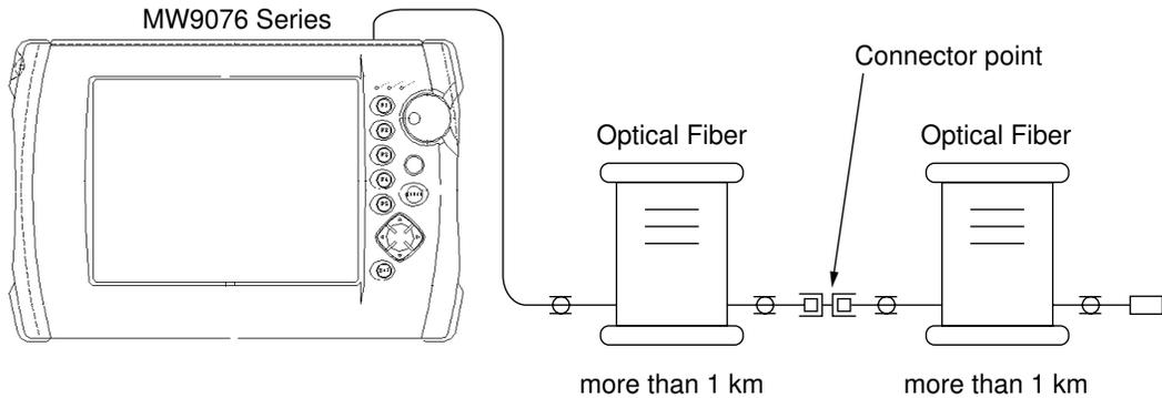
The maximum cable length in this setup is 10 km.
