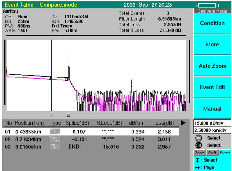
To turn off the waveform comparison function, press **Menu** to open the menu window. Select “Application” using **^**, **v** keys. When “Application” is selected, “Compare off” is displayed on the F1 function key label. Pressing **F1** (Compare off) turns off the waveform comparison function.
