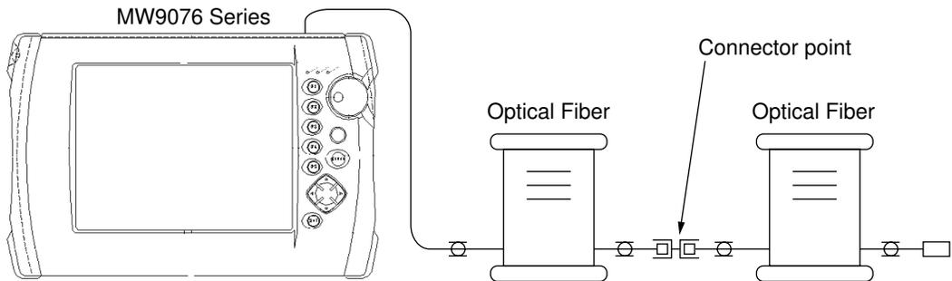
The maximum cable length in this setup is 10 km.
