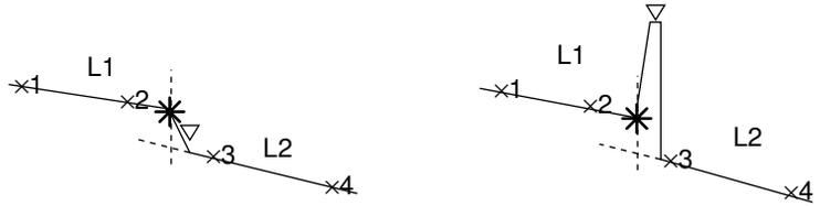
There are two methods for determining these lines: the LSA and 2PA methods. Of these methods, this section explains the LSA (Least Square Approximation) method.
