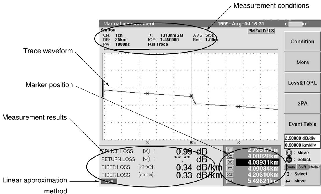
Six markers and the measurement results of splice loss and return loss are displayed on this screen. In addition, the following items are displayed.
