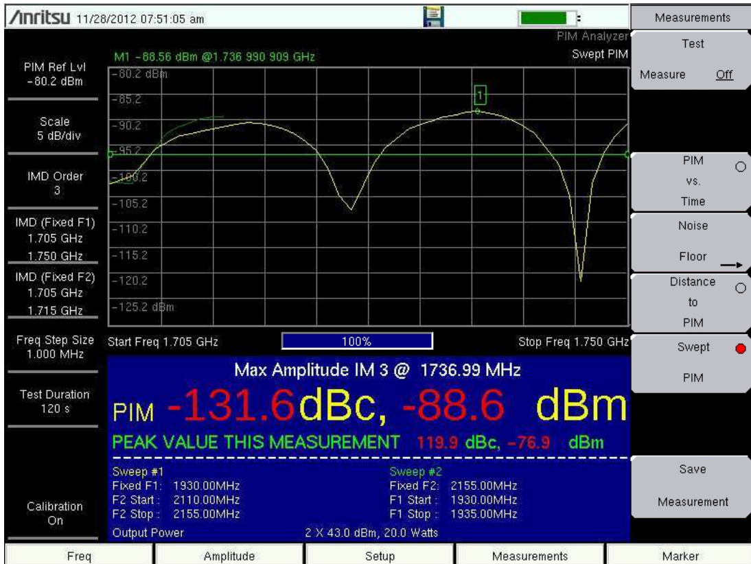
Figure 11-4. Swept PIM IM3 Measurement
