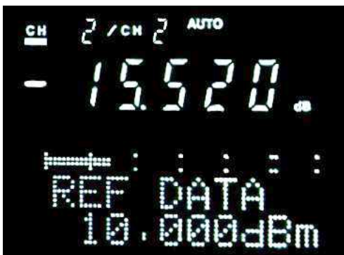
Measurement Relative to Reference Data (MT9810A display)
