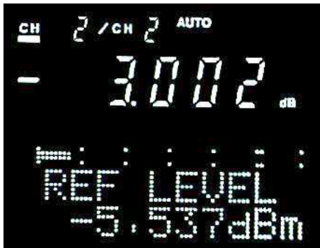
Optical Insertion Loss Measurement using Relative Value (MT9810A display)
