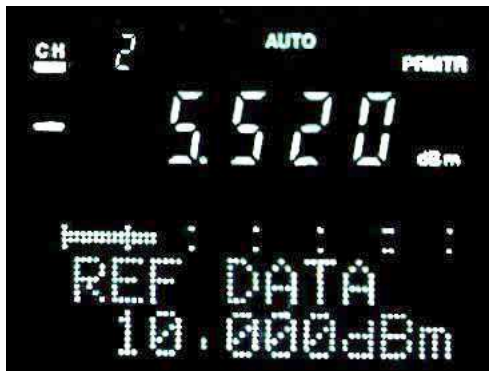
Reference Data Input (MT9810A display)
