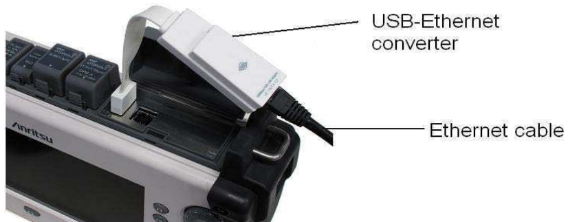
Figure 14-2: Ethernet Cable Connection
