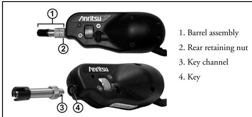
Figure 11-6: Attaching a Probe Tip with Optics
