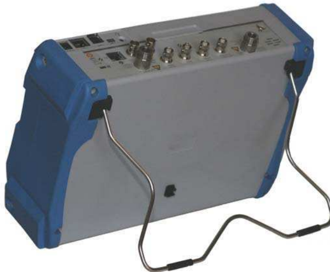
Figure 1-4. Tilt Bail Extended
