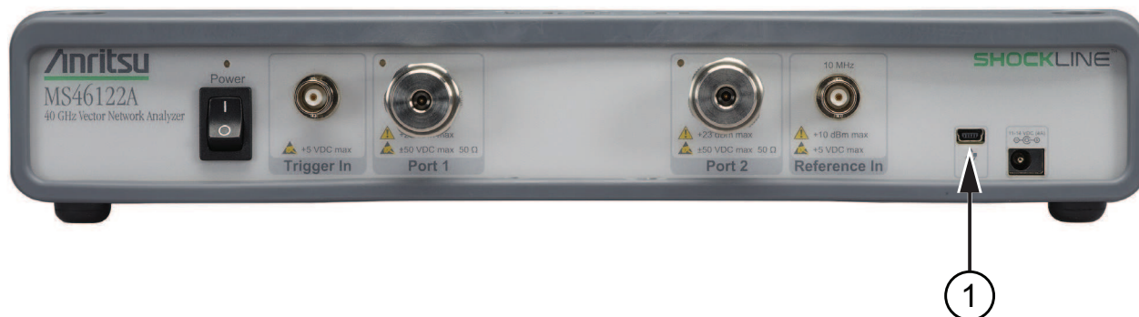
Figure 2-4. ShockLine MS46122A Series VNA USB Connection
