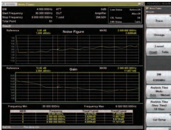
Measurement Result: Example of Graph display (Frequency Mode: Sweep, Screen Layout: Graph)
