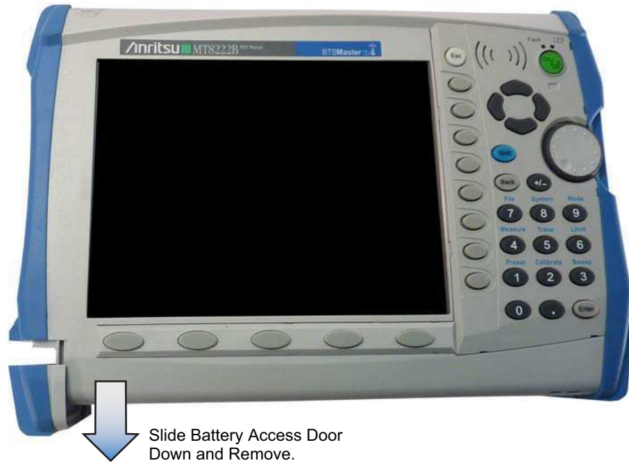
Figure 4-3. Removing the Battery Access Door
