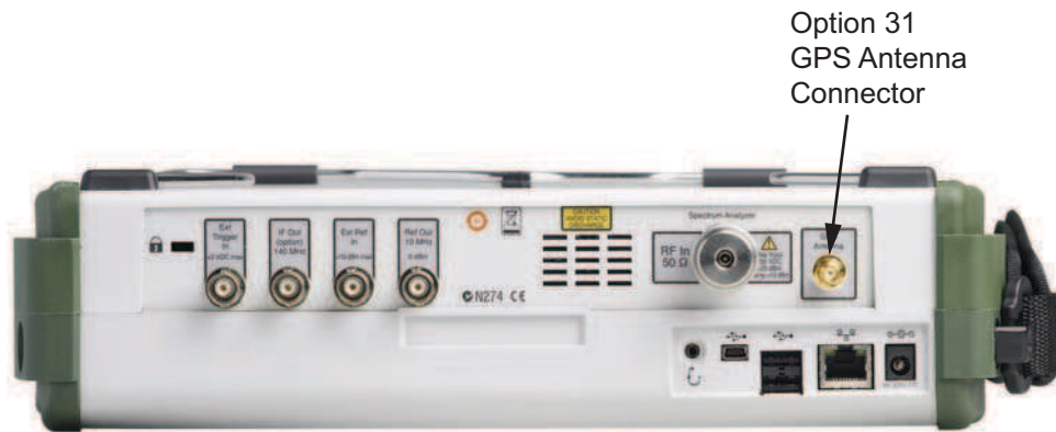
Figure 5-1. Remove Option 31 Lock Nut and Washer
