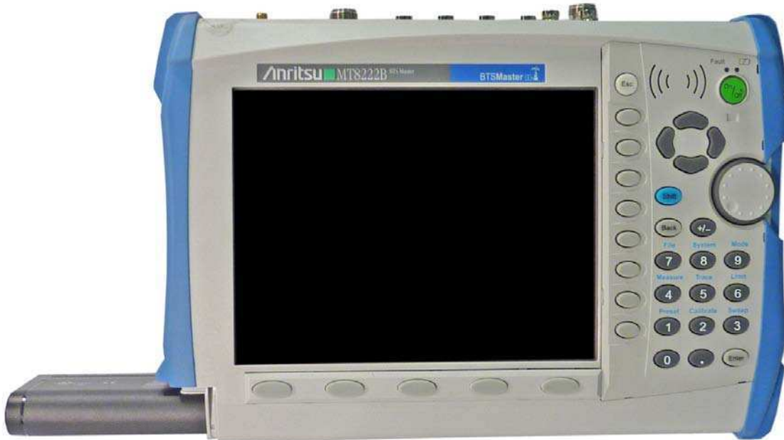
Figure 4-4. Removing the Battery
