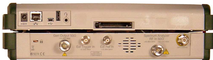
Figure 4-6. Separate the Two Halves of the Case
