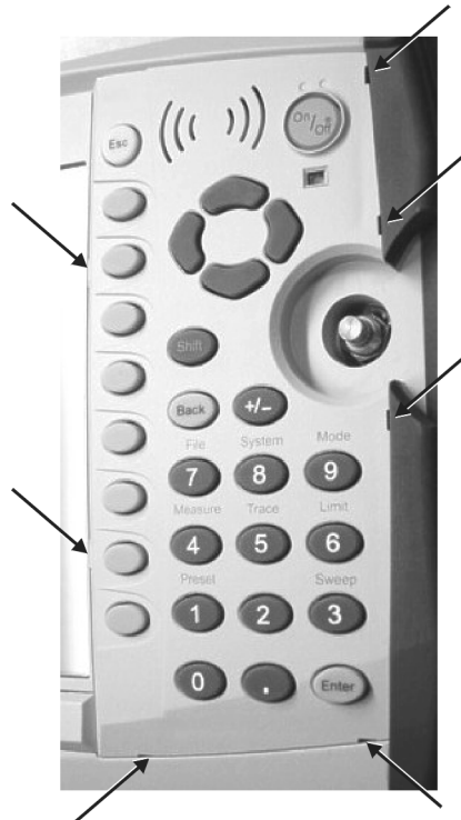
ARROWS POINT TO FRONT BEZEL LOCKING TAB LOCATIONS
