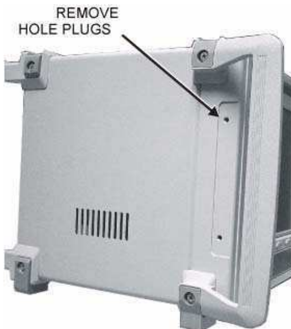
Figure 1-2. Rack Mount Bracket Mounting Holes
