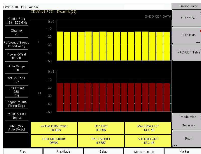
Figure 13-6. EVDO CDP Data Measurement Display
