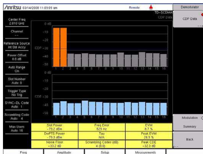
Figure 14-4. Demodulator Measurement – CDP Data
