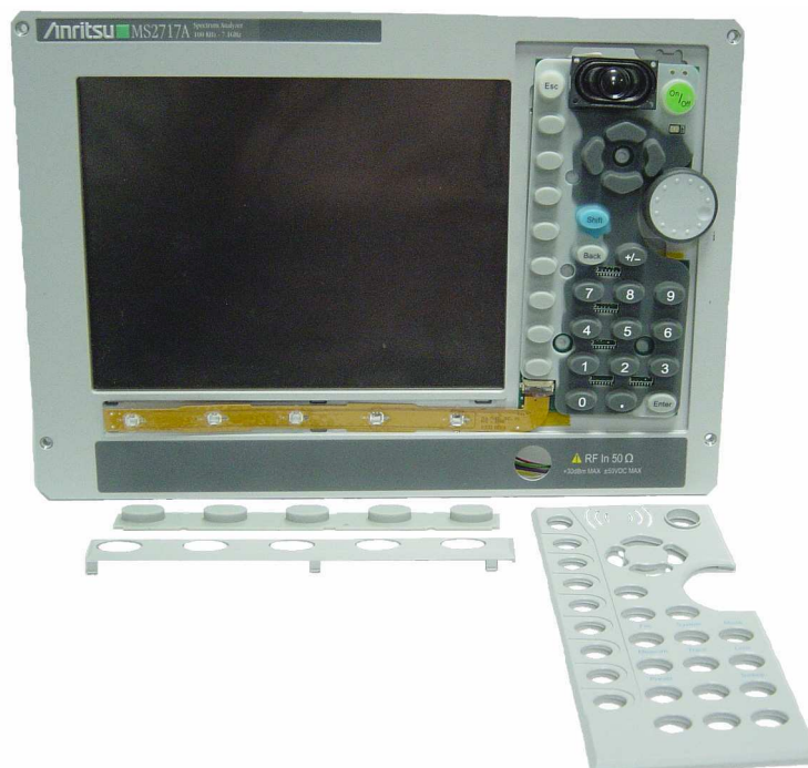
Figure 4-32. Keypads and Bezels, Front Panel
