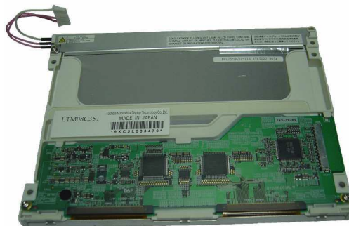
Figure 4-25. LCD Display with Backlight Attached
