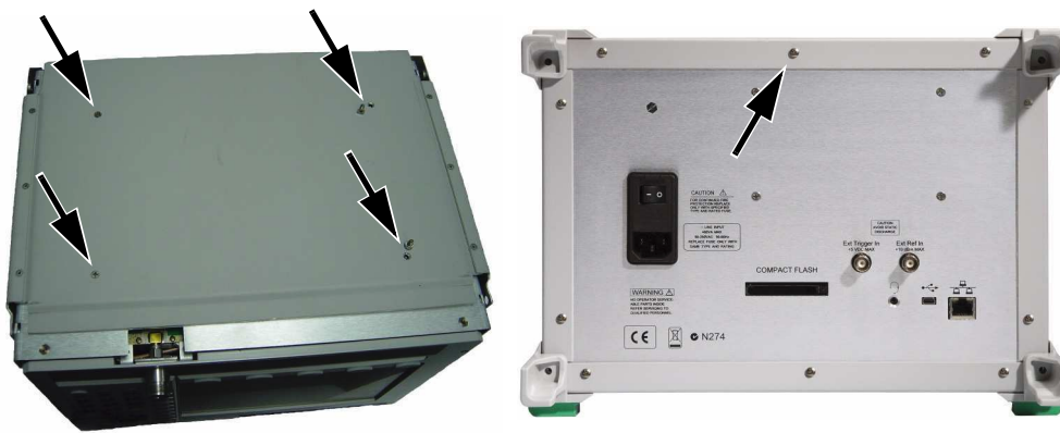
Figure 4-7. Screws that Hold Chassis within Outer Enclosure
