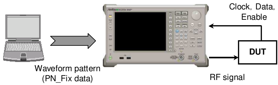
Fig. 3.8-6 BER measurement using PN_Fix data
