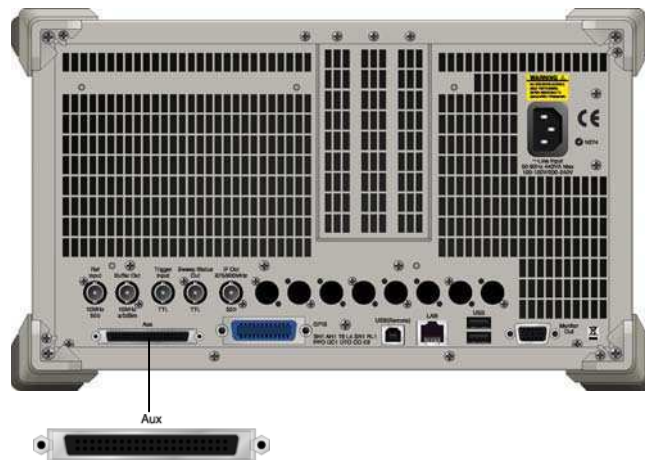
Fig. 2.6.3-1 Connector connection location
