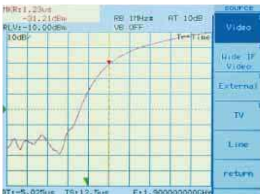
High-speed time-domain measurement (TS = 12.5 \mu s)
