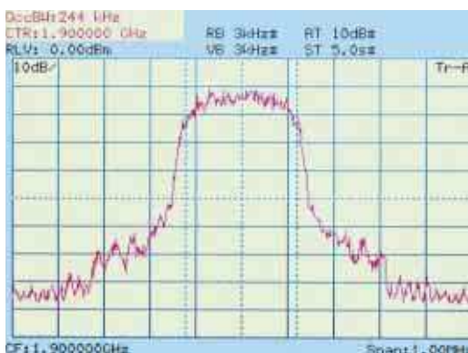
Occupied bandwidth measurement
