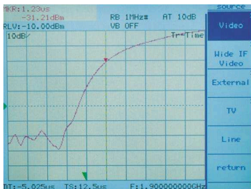
High-speed time-domain measurement (TS=12.5 \mu s)
