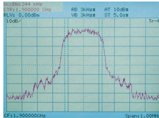
Occupied bandwidth measurement
