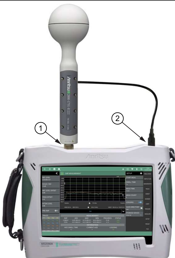
Figure 3-53. Isotropic Antenna Connection
