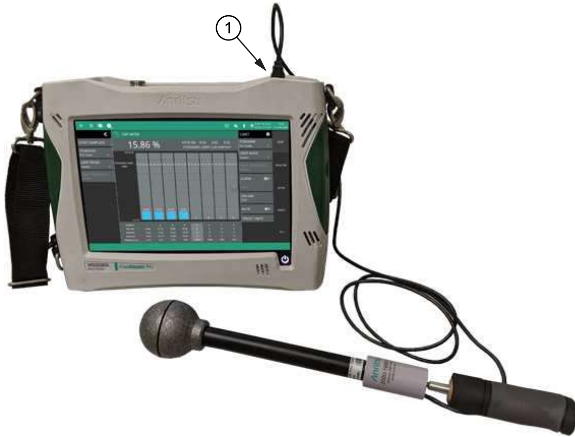
Figure 8-2. EMF Meter Probe Connection
