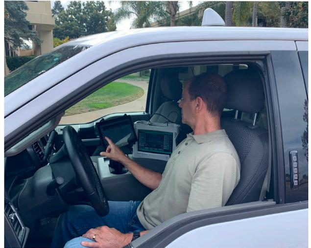
MIH system installation with large in vehicle display and omni antenna on roof
