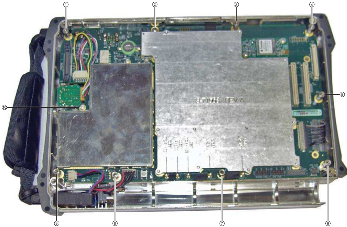
Figure 7-20. Main PCB (Mother Board) in Case – Standoffs and Screws
