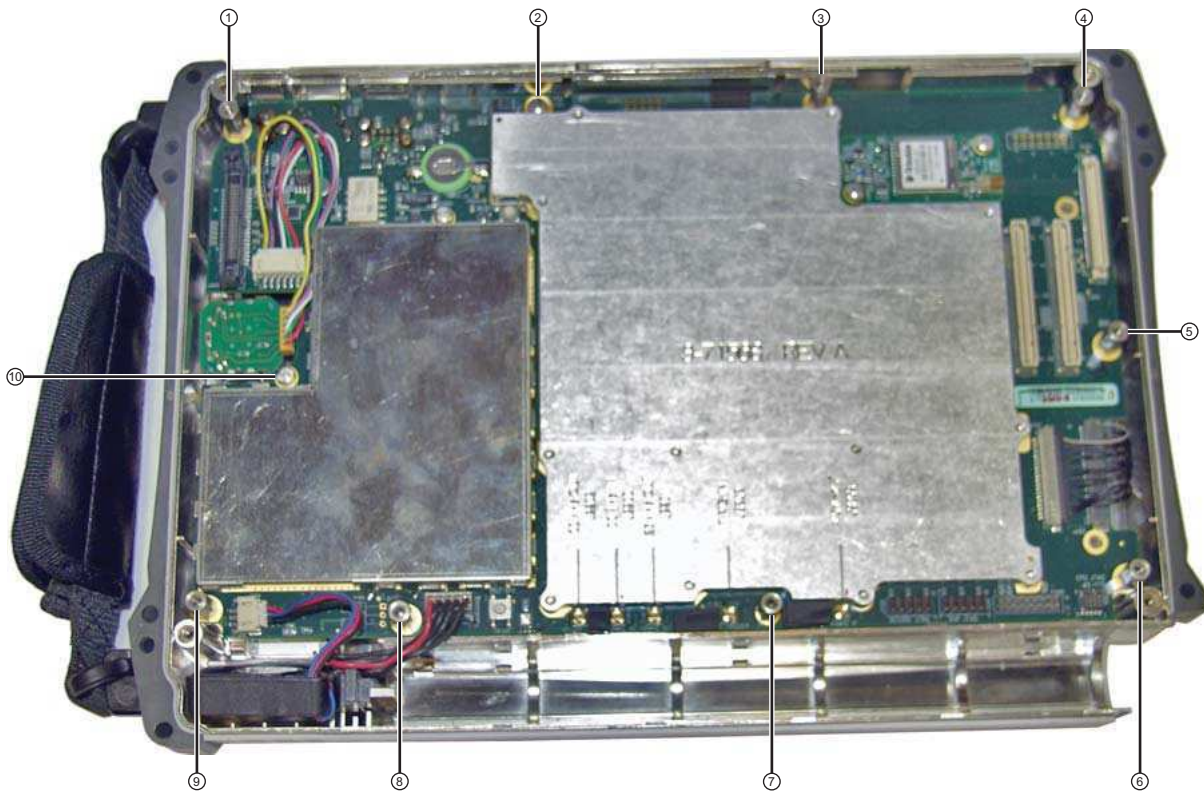
Figure 7-27. Main PCB (Mother Board) in Case – Standoffs and Screws
