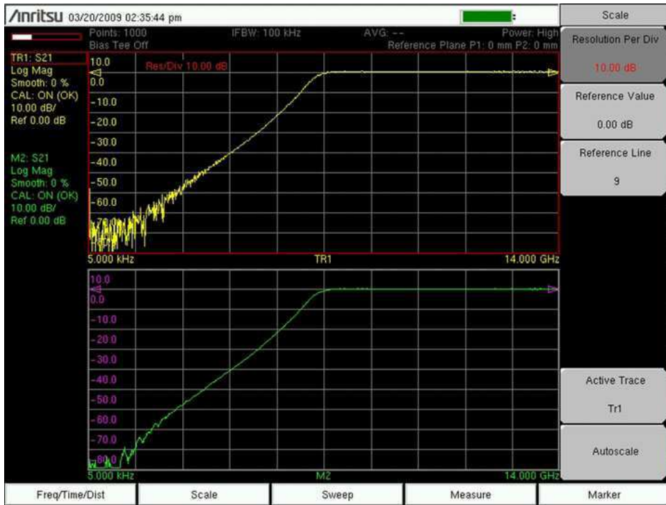
Figure 5-7. 100 Hz (top trace) and 100 kHz IFBW
