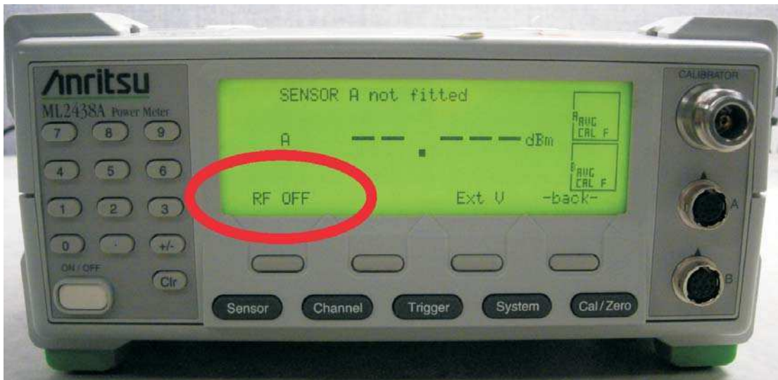
Figure 2-21. ML243xA Power Meter
