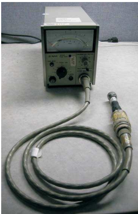
Figure 2-17. 432A Power Meter
