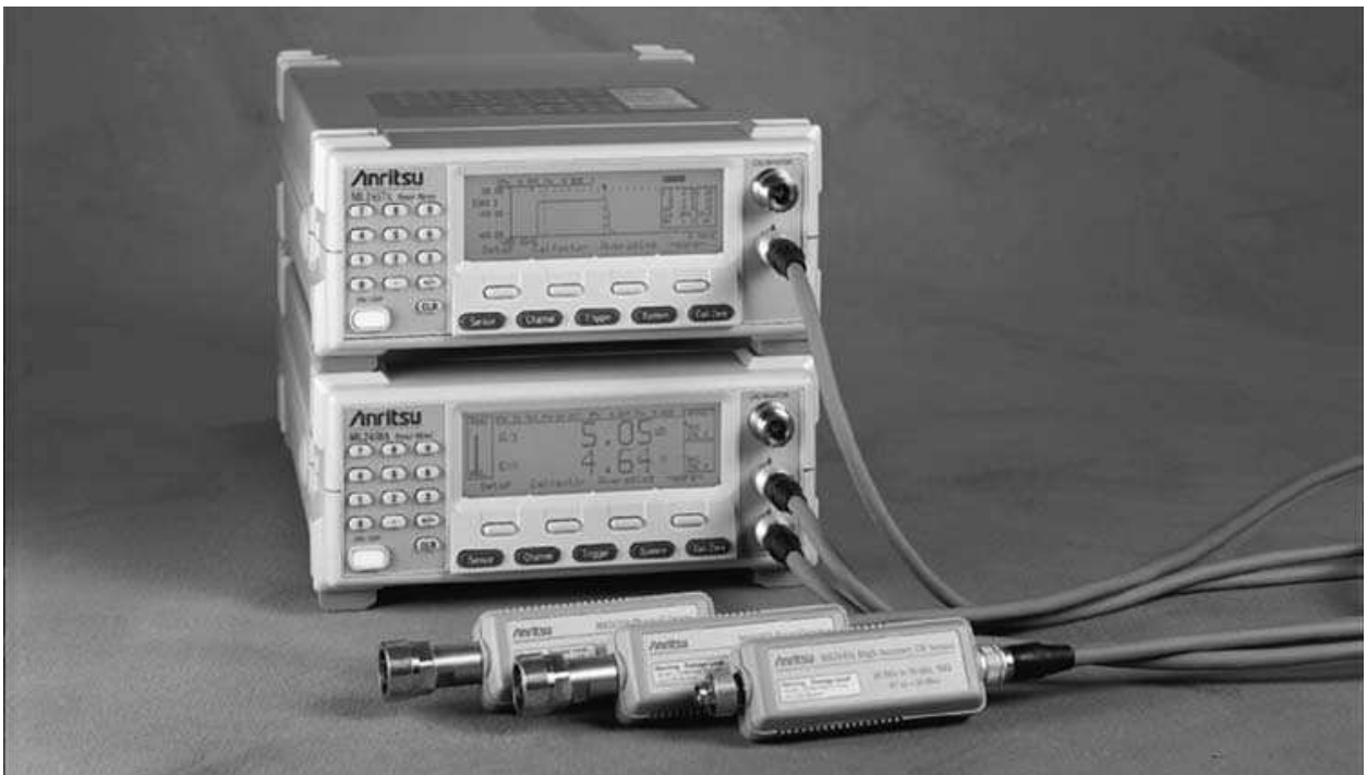
Figure 1-1. ML2430A Series Power Meters
