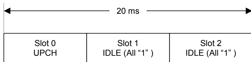
Downlink UPCH 1-slot transmission (DL_Packet_Slot_0)
