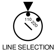
Figure 2-7. LINE SELECTION Setting (Network Analyzer)
