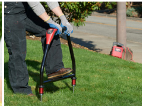
Pinpoint fault location by using the AF-600 with the UAT-600 Transmitter
