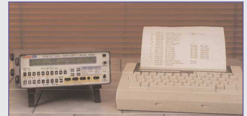
AM8a and printer with printout showing SLC®96 channel assignment.
