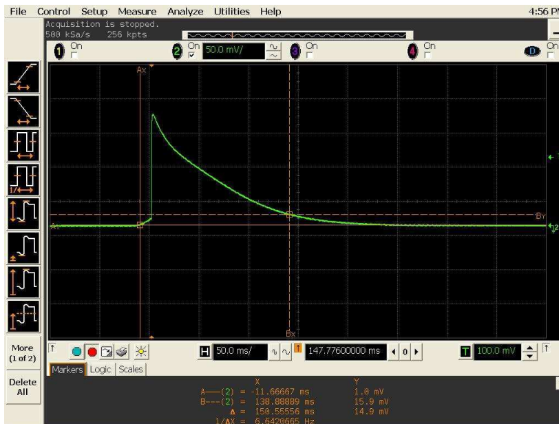
Figure 5-13 Load transient response time
