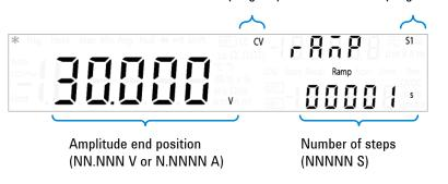
CV/CC ramp signal parameters Ramp signal range
