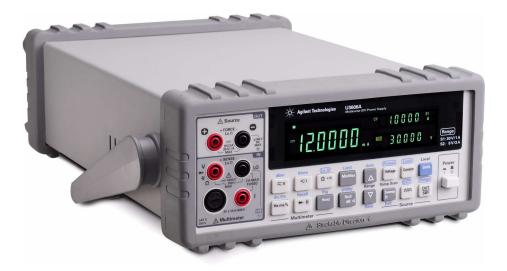
The Agilent U3606A Multimeter | DC Power Supply unit is a combination of a 5½ digit, 120000 count digital multimeter and a 30 W DC power supply with a square-wave generator, that is able to work simultaneously and independently.
