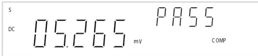
Figure 2-5 Typical Comp operation display
