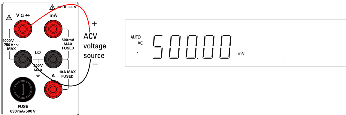
Figure 1-10 ACV terminal connection and display
