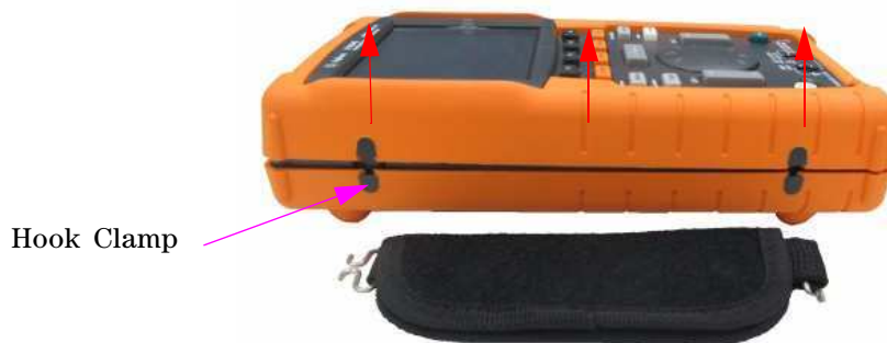
Figure 8-8 Remove handler from the instrument
