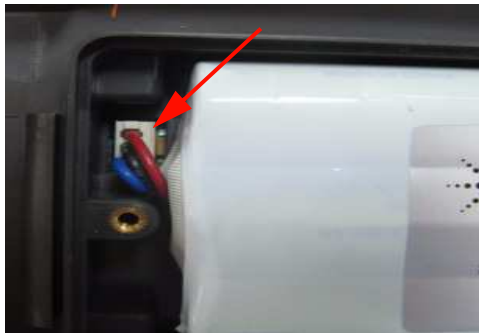
Figure 8-4 Unplug 3-wire connector from PCBA board using tweezer
