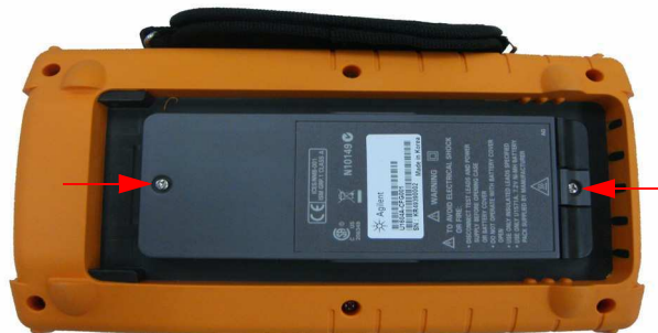
Figure 8-3 Remove battery cover screw
