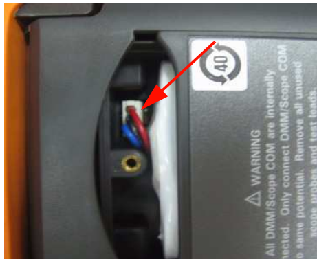
Figure 8-6 Unplug 2-wire connector with a tweezers.
