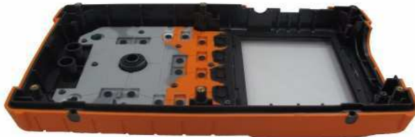
Figure 8-12 Remove keypad from the front cover
