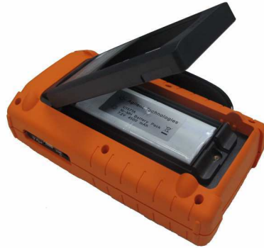
Figure 8-5 Remove battery pack cover without removing stand
