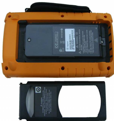
Figure 8-2 Disassemble the stand from the instrument
