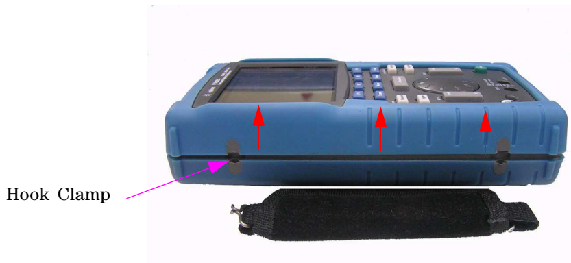
Figure 8-8 Remove handler from the instrument
