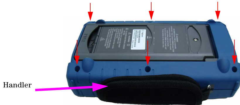
Figure 8-7 Remove screw from the rear cover
