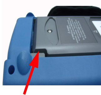
Figure 8-1 Push towards the arrow direction to remove the stand
