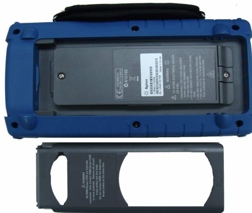
Figure 8-2 Disassemble the stand from the instrument
