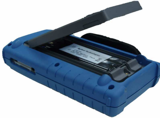
Figure 8-5 Remove battery pack cover without removing stand
