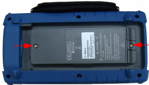
Figure 8-3 Remove battery cover screw
