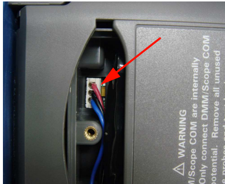
Figure 8-6 Unplug 2-wire connector with a tweezers.
