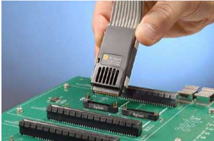
Figure 11 Connecting Midbus Probe Tip
