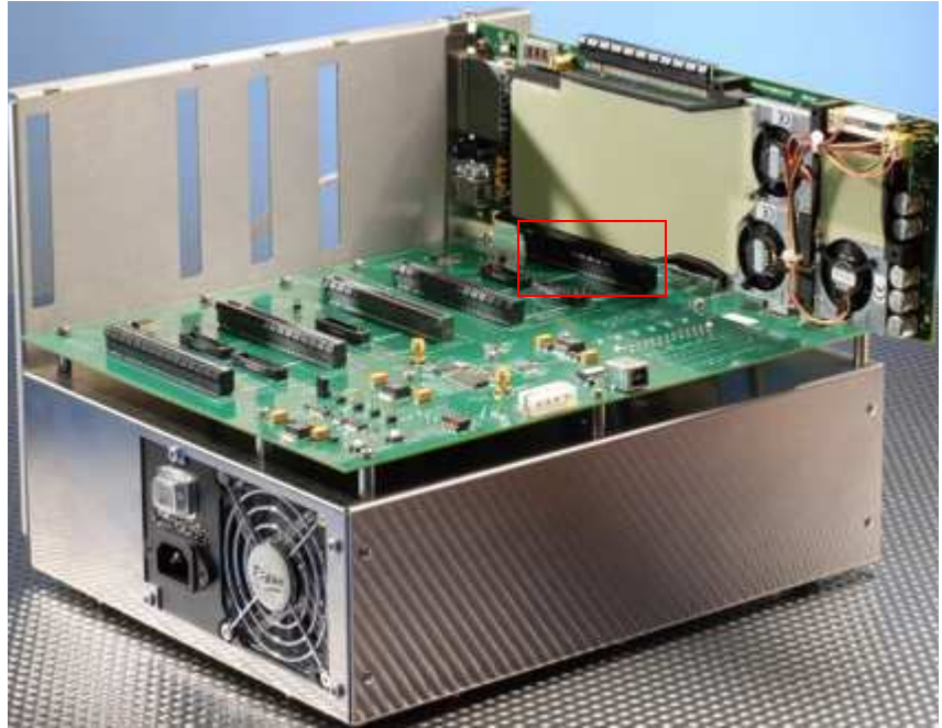
Figure 5 Exerciser Card mounted on N5316A Test Backplane
