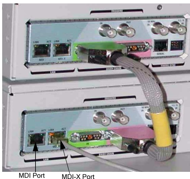
Figure 9 Interconnection between the Master and Slave Chassis
