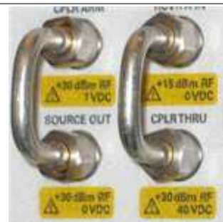
Re-configure the receiver port front-panel loops to a vertical orientation.
