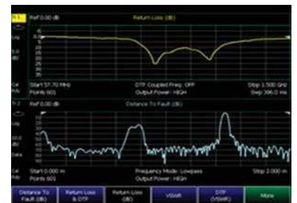
View return loss and DTF simultaneously
