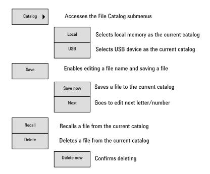
**Catalog** Pressing this softkey selects the catalog for storing configuration files. **Local** means saving a configuration file in the instrument's internal memory. **USB** means saving a configuration file to a USB memory stick by way of one of the USB device type connectors. Insert a external memory stick into the USB connector
