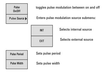
**Pulse On Off** Press this softkey to enable the pulse modulation. The PULSE annunciator will then be displayed. The RF carrier will be modulated only when the Moder hardkey is pressed and the Moder annunciator displays.
