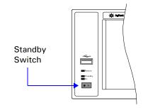
Pressing this front panel switch toggles power to the signal generator between on (green LED on) and standby (orange LED on). In standby mode, the signal generator is switched off, however the instrument is still connected to the line power. The rear panel line switch and the detachable power cord are the instrument disconnecting device. The front panel standby switch, therefore, is not, and should not be used as a power switch.
