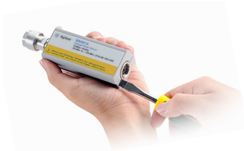
Figure 3-2 Removing power sensor shell
