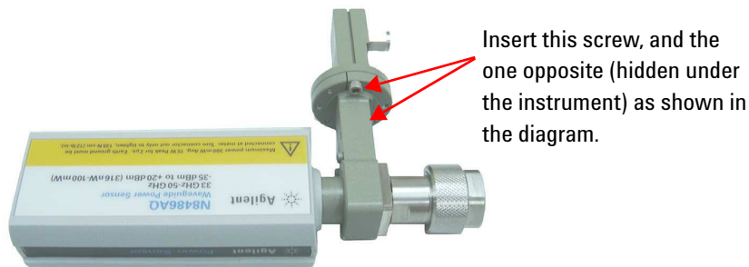
Figure 1-3 Connecting waveguide flange to the N8486AQ power sensor
