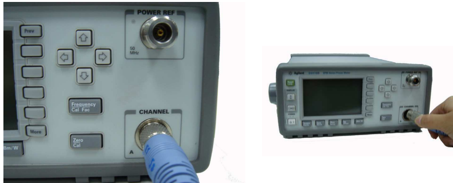
Figure 1-2 Connecting a sensor cable to power meter
