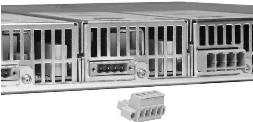
Figure 5. Quick disconnects for power and sense leads
