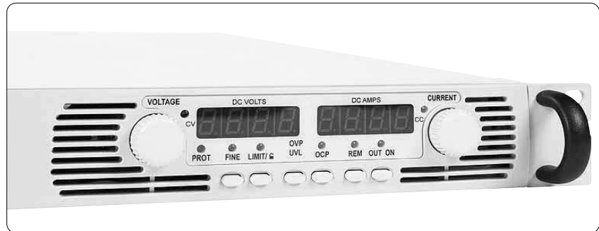
Figure 1. Front-panel control knobs and buttons make it easy to use N5700 power supplies.
