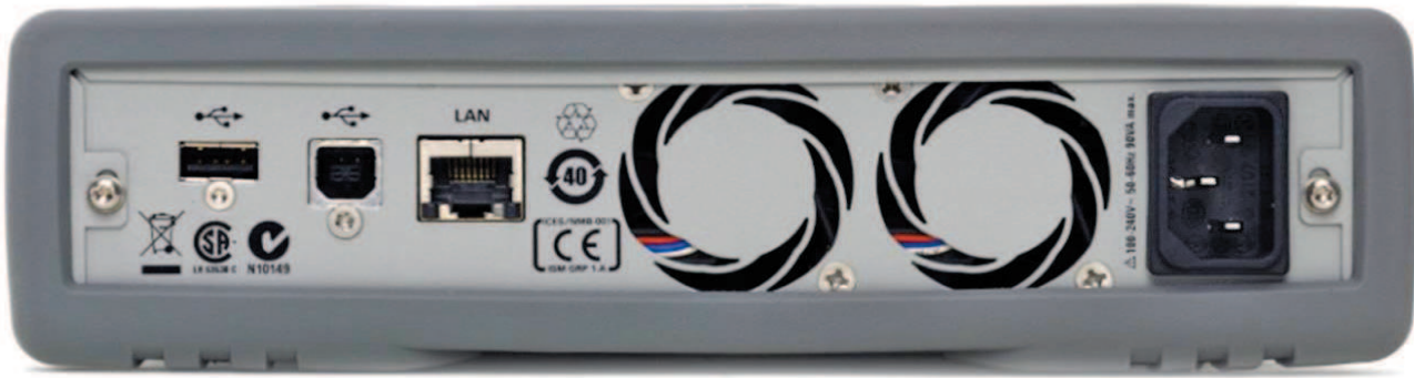
Figure 8. USB and LAN connection are located at the back of the Keysight N4877A clock data recovery and demultiplexer 1:2.
