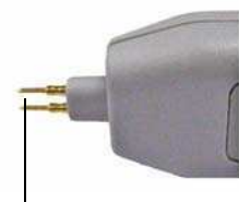
Two single signal pins inserted into probe
