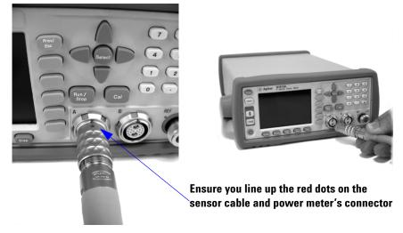
Allow a few seconds for the power meter to read the data contained in the power sensor's EEPROM.
