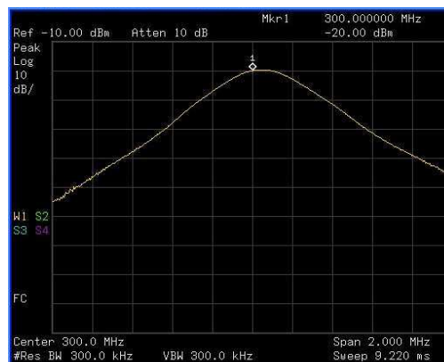
Figure 3-5 Unresolved Signals of Equal Amplitude
